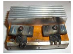
Damage from high current to the heat sink and IGBTs
