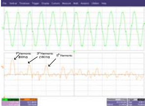
210v input with a 50ohm load distorted sine wave (top), frequency analysis (bottom)
